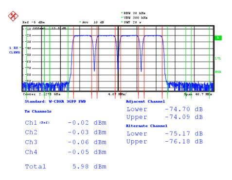
Figure 3: High dynamic four channel 3G multicarrier signal
