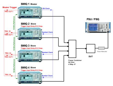
Figure 1: Hardware test setup for multi carrier generation
